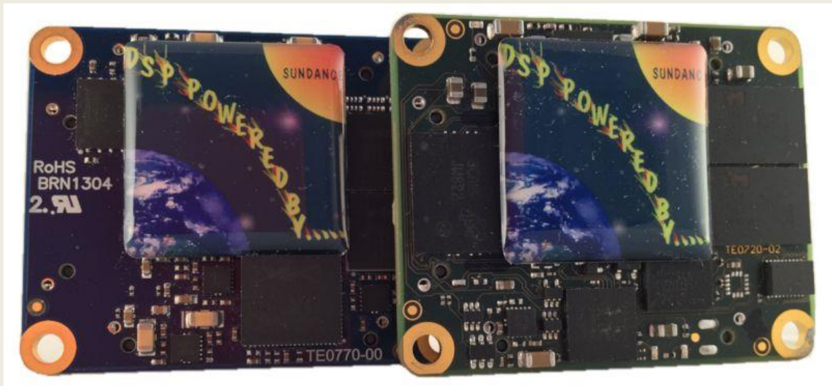
Figure 1: The 40mm x 50 mm SoM Module for EMC 2 with Xilinx Artix-7 FPGA
