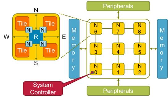
Fig. 1: Configuration of the reference network[?]
