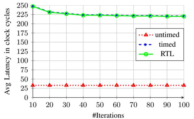
Fig. 8: Avg. flit latency in a 64 router NoC
