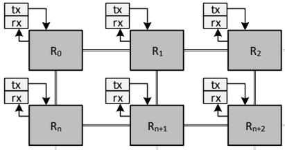
Fig. 6: 2D mesh NoC topology test configuration with traffic generators and receivers
