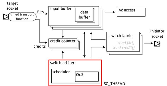
Fig. 4: Router architecture of the timed simulation model
