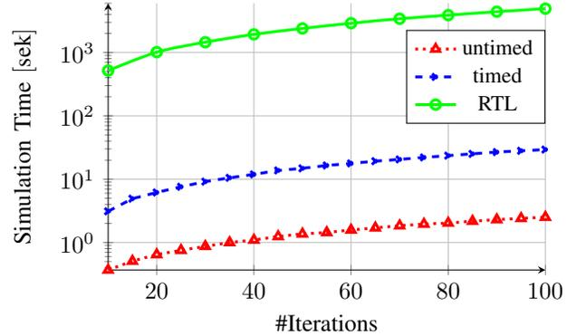
Fig. 7: 64 router NoC simulation speed (logarithmic) of timed, untimed and RTL models
