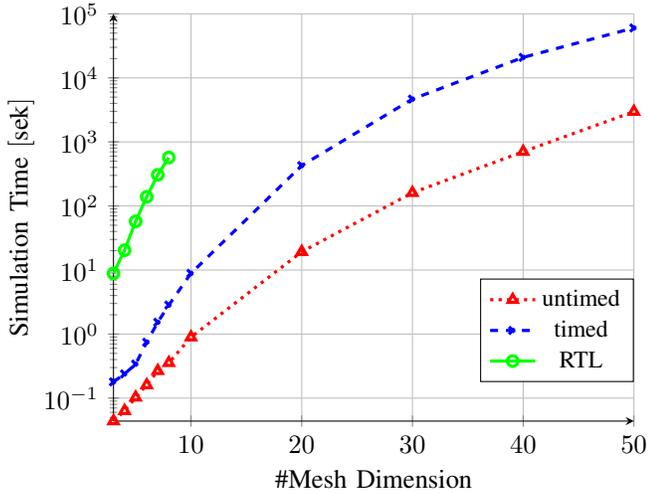
Fig. 9: 9 - 2500 router NoC simulation speed (logarithmic) of timed, untimed and RTL models (RTL model supports up to 8x8 routers)
