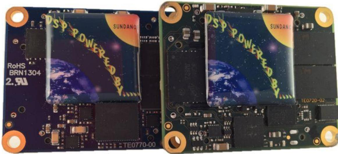
Figure 5: The 40mm x 50mm SoM Module for EMC<sup>2</sup> with Xilinx Zynq SoC, Artix-7 or Kintex-7
