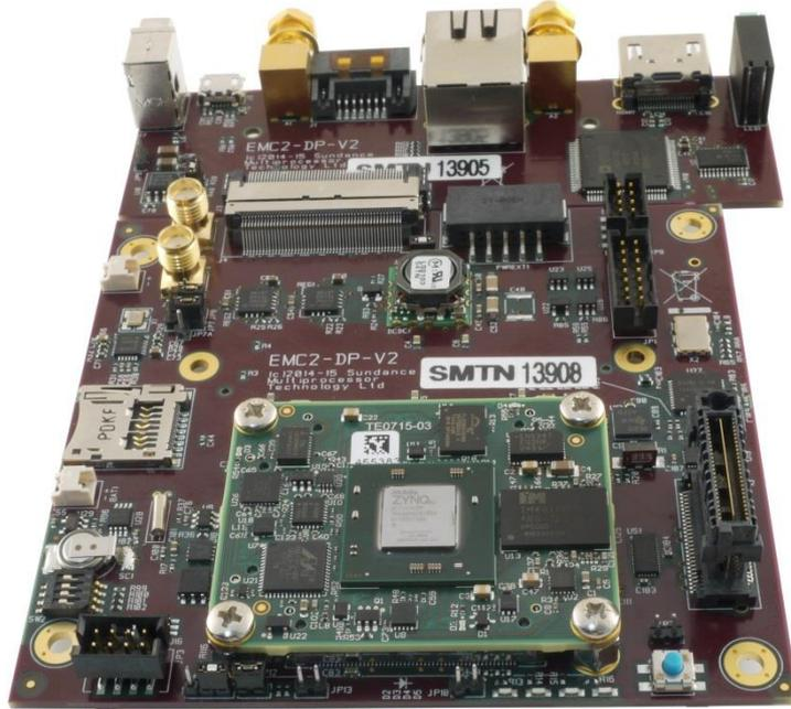
Figure 1: The EMC<sup>2</sup> showing the Stackable PCIe/104 OneBank Connector and the Cable-less I/O board
