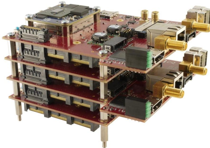
Figure 2: EMC<sup>2</sup> stacked, using the PCI Express Lanes, to provide 8x ARM9 CPU Cores
