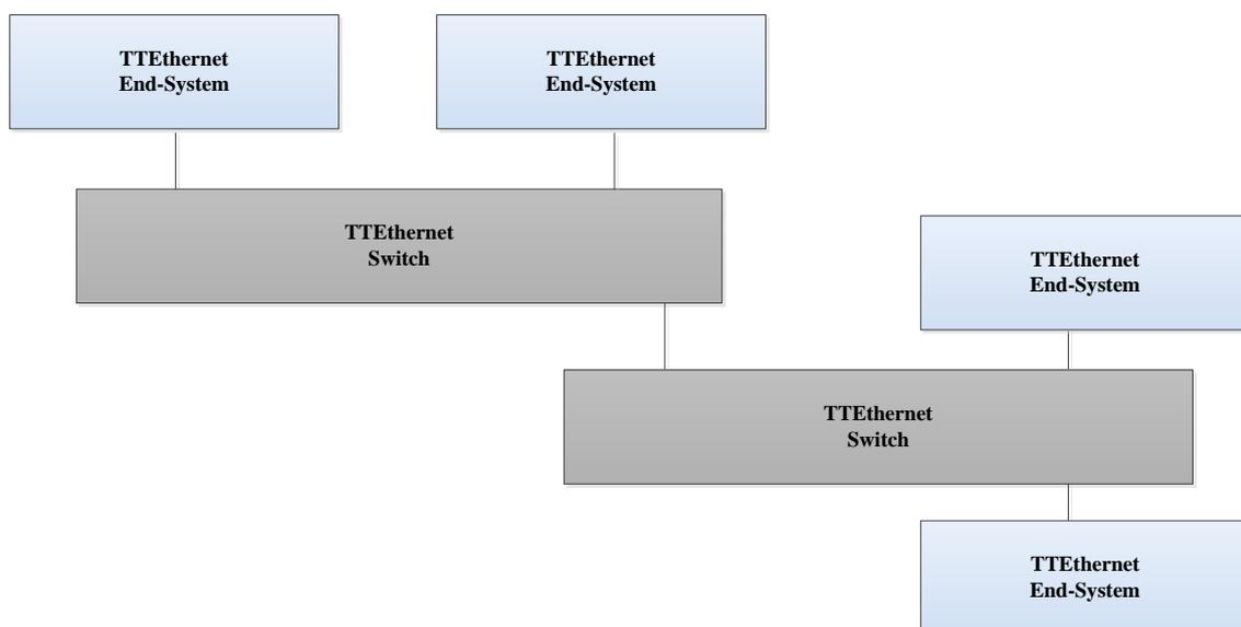
**Figure 6: Simple TTEthernet network with 2 switches and 4 end-systems**
