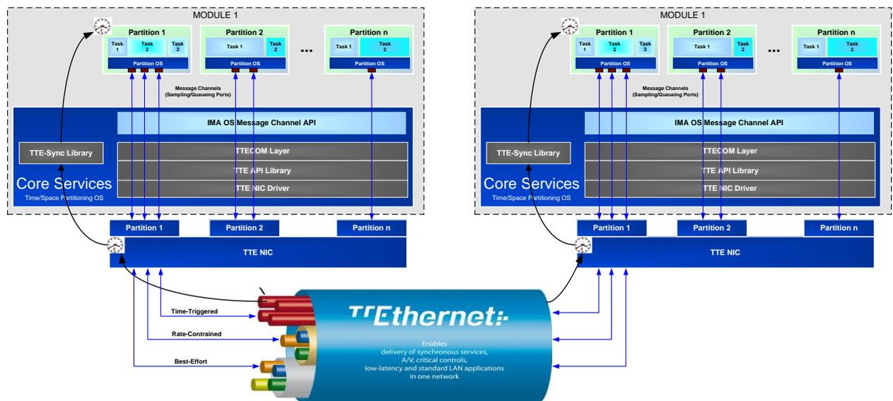
**Figure 10: Distributed partitioned architecture**
