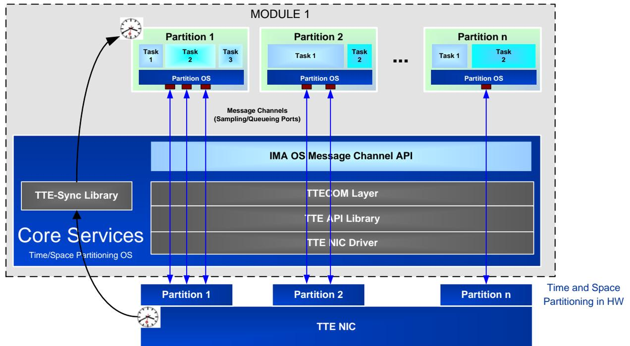
**Figure 9: TTEthernet SW stack integration**
