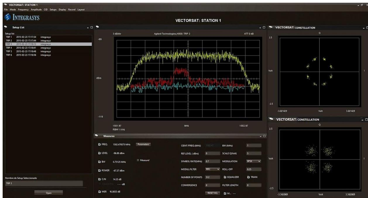
Figure 26: Vectorsat Client demodulating an 8-PSK carrier with interferences
