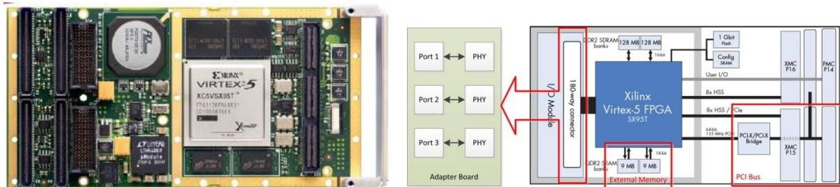
Figure 11: ES Virtex-5 evaluation implementation on XMC-FPGA05D
