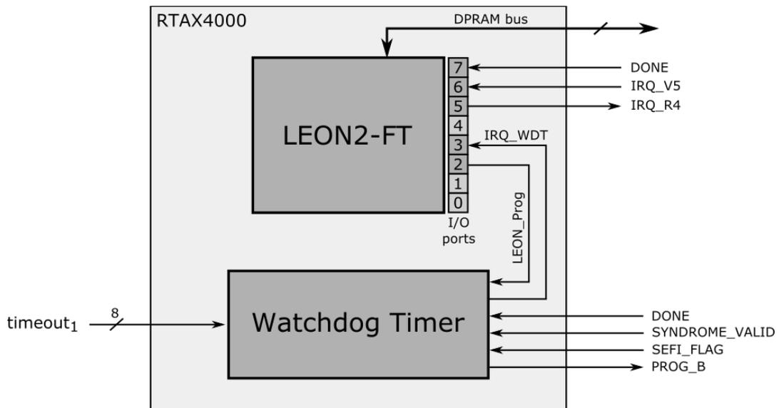
Figure 3: Modules implemented in RTAX4000 device
