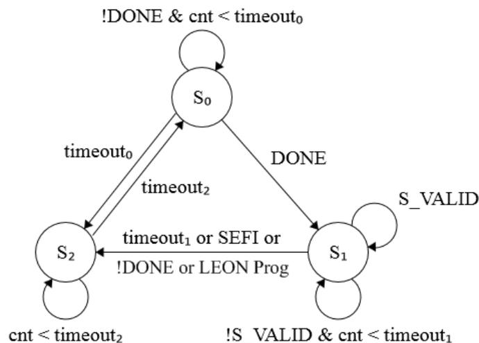
**Figure 4: FSM diagram of Watchdog Timer**
