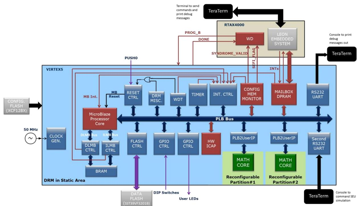
Figure 2: System architecture diagram of the Reliable and Self-Healing DRM
