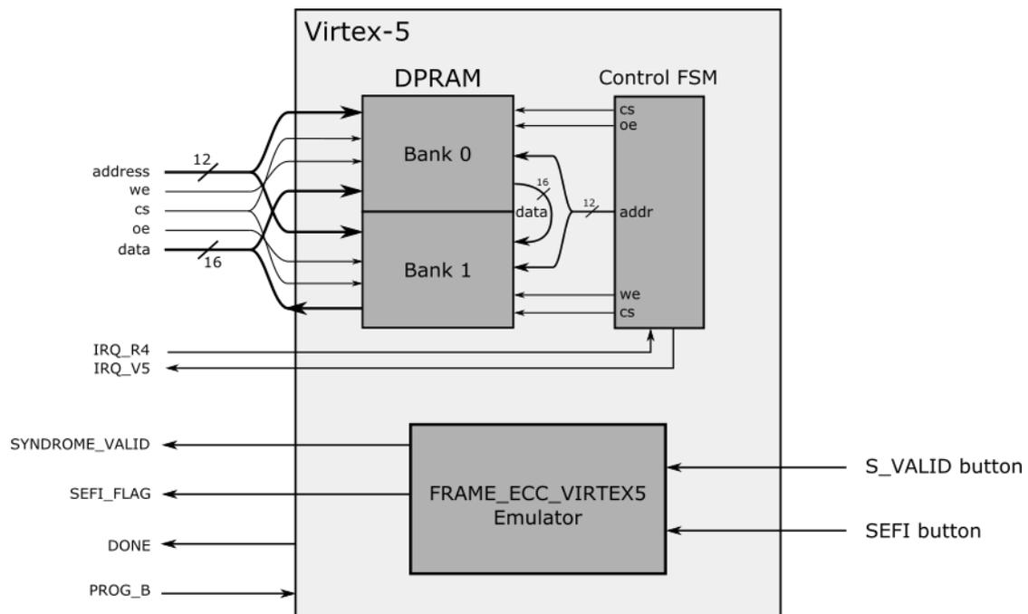
Figure 5: Modules implemented in Virtex-5 to validate the design
