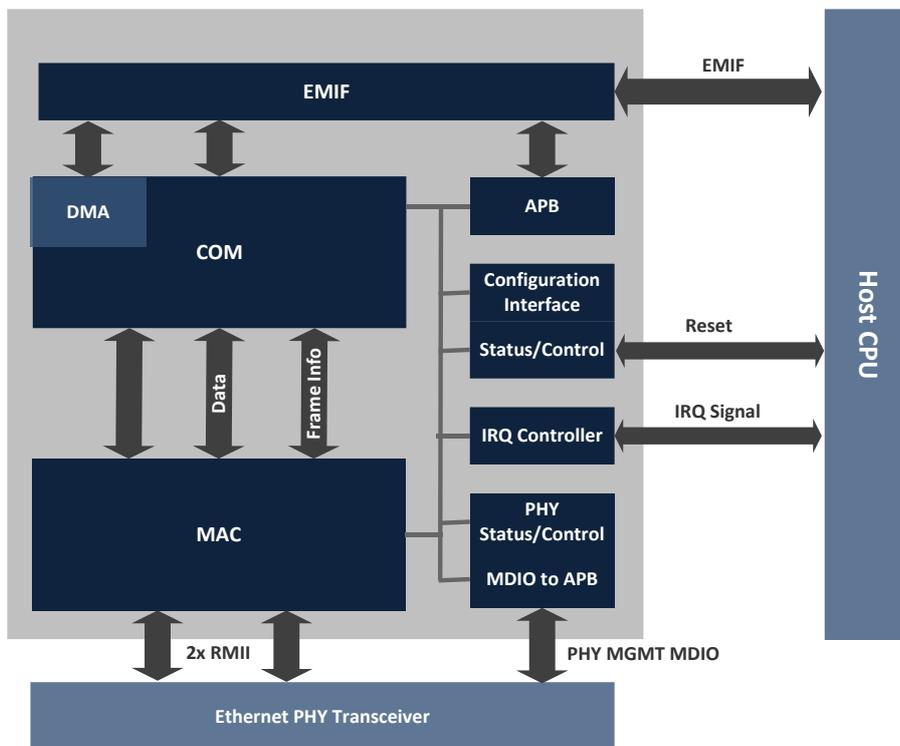
Figure 8: Schematic overview of the Network ES Controller
