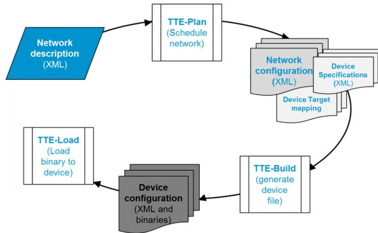
**Figure 21: Network configuration toolchain**
