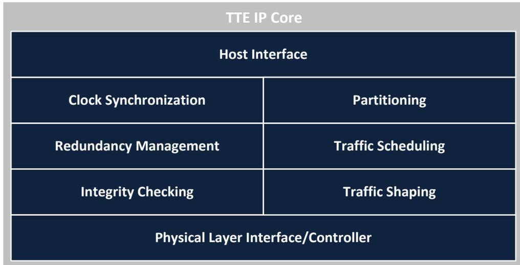
Figure 7: Services of the TTEthernet network controller
