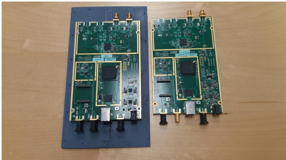
Figure 25: USRP B200 Transmitter and Receiver
