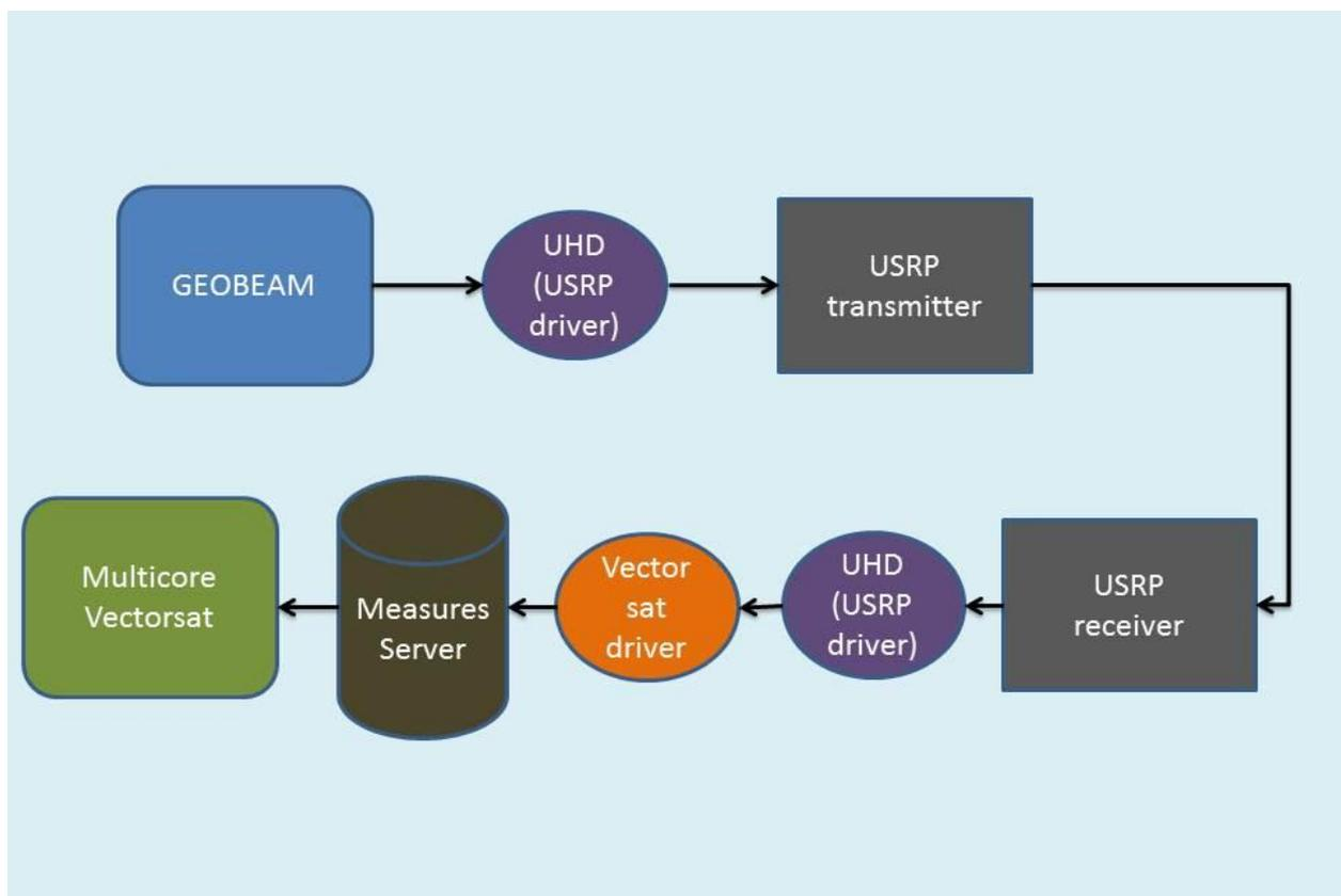
**Figure 22: Satellite Communications Link Emulator Block Diagram**
