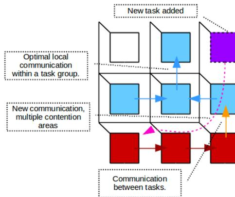
**Figure 2: 3x3 mesh network example with potential communication contention**
