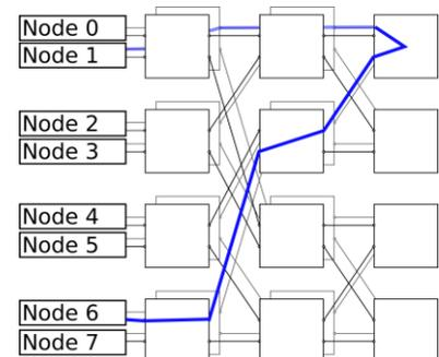
**Figure 34: The same network, folded and depicting node connections**
