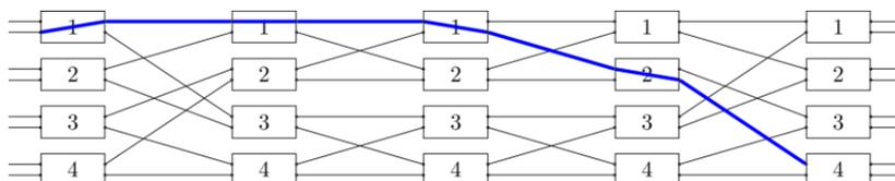
**Figure 18: A five-stage, eight-port network with a single route highlighted**
