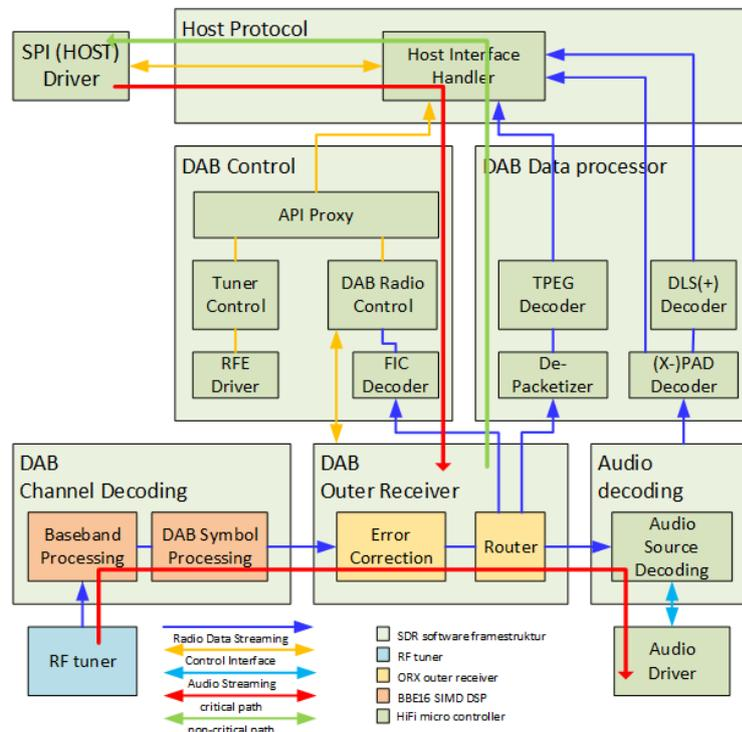
**Figure 80: simplified structure of a DAB+ receiver**
