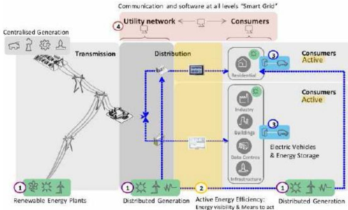
**Figure 7: Smart Grid concept**
