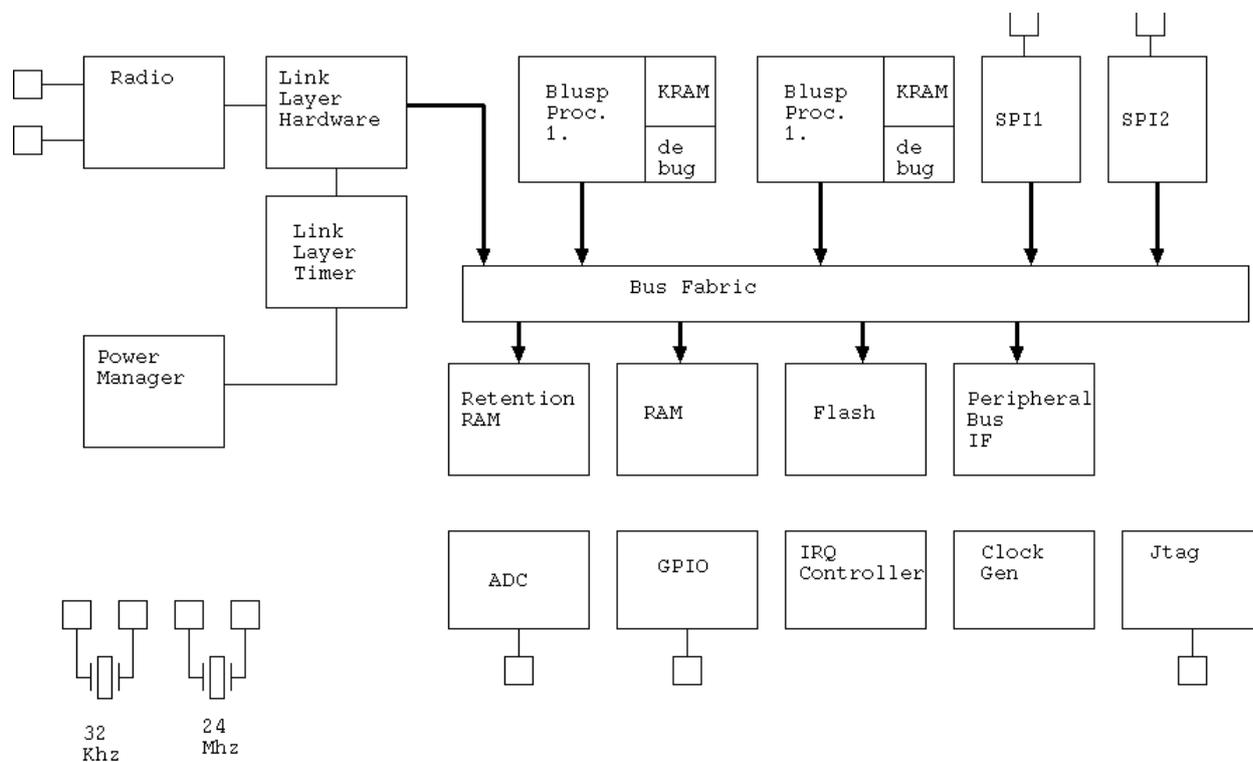
**Figure 6: Demonstrator block diagram**
