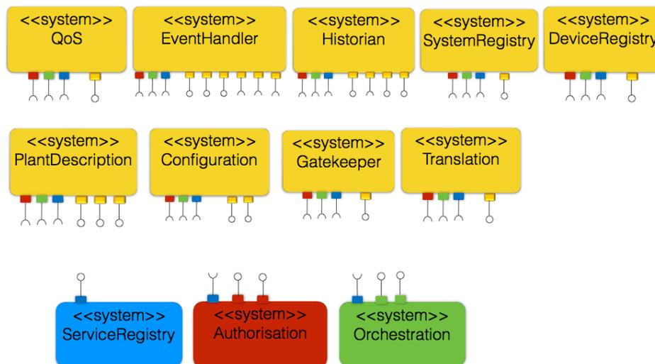
**Figure 2:** Mandatory core and Support Systems of the Framework.
