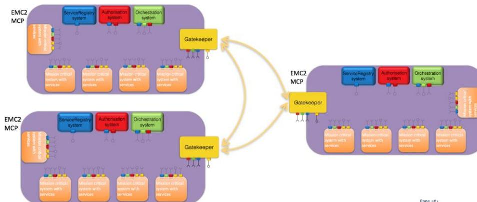
Figure 1: Local clouds in an MPSOC setting.
