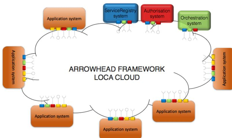
**Figure 3:** A collection of applications with a minimum but mandatory middleware forming a local cloud.
