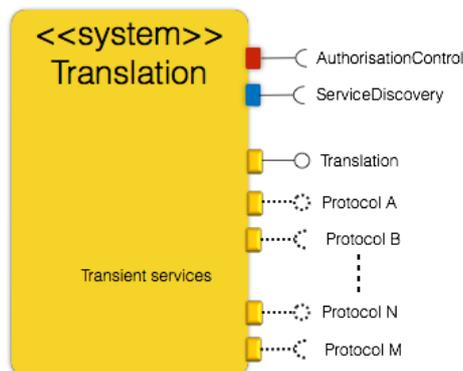
**Figure 7:** The Translator system and its produced and consumed services.
