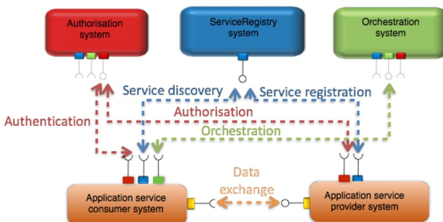
**Figure 4:** Minimal local cloud with indications of mandatory core service interaction enabling service exchange between two application systems.
