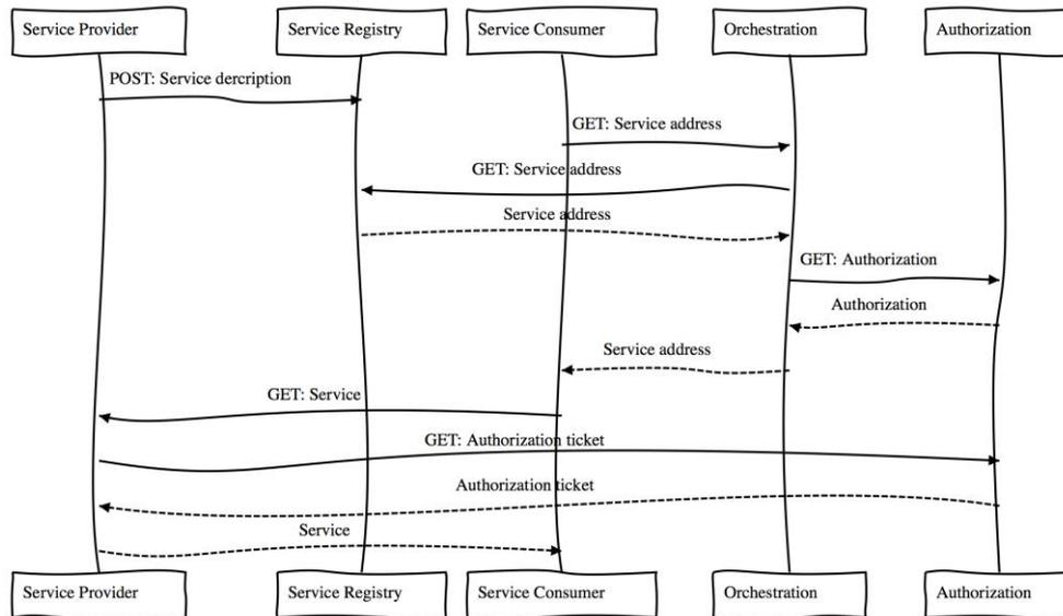
**Figure 5:** Simplified sequence diagram example of messages exchange in an Arrowhead Framework Local Cloud.
