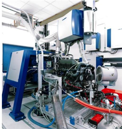
Figure 19: Engine Test Bed
