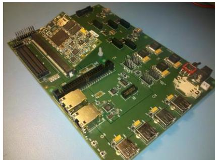
Figure 24: Photo of demonstrator carrier board and module
