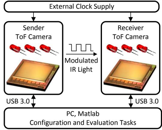
Fig. 3. The design principle of our proof-of-concept prototype.
