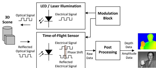
Fig. 2. The concept of PMD-based Time-of-Flight 3D sensing, obtained with changes from [3].
