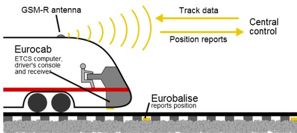
Fig. 4. ETCS Level 3 schematic [37]
