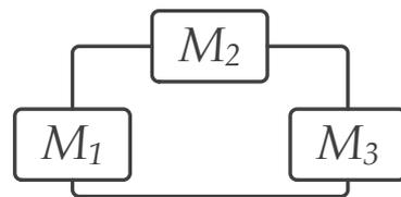
Fig. 2. Triple Modular Redundancy communication: The modules exchange messages with each other in order to detect errors, maintain a global time and reach a consistent agreement of states among the replicated modules (i.e., *interactive consistency* [18]).
