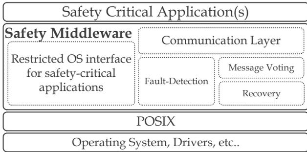
Fig. 1. Layered architecture of the *TAS Platform* [8]: Safety-critical applications gain access to system resources through a middleware layer, which transparently provides the services required to operate within the restrictions of a safety case for the application.
