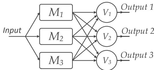
Fig. 3. TMR System with distributed voters: A distributed majority voting function is used in order to unify the states of the different processors [18] [20] and produce a single correct output (a comprehensive survey of different voting algorithms can be found in [21]).
