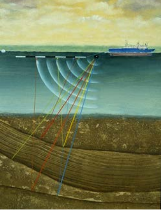
Fig. 4 Reflected waves from shock events illustrating the huge amount of data provided in these kinds of experiments
