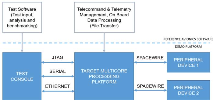
The platform management presents specific requirements of reliability, robustness, as well as various levels of criticality and dependability both at software and hardware level. The use of hypervisors and paravirtualization techniques is considered as a feasible way to deal with these requirements.
