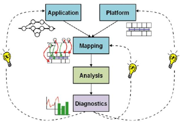
Design-space exploration typically involves the co-development of an application, a platform, and the mapping of the application onto the platform. Diagnostic information is used to (semi-automatically) improve application, platform, and/or mapping.
