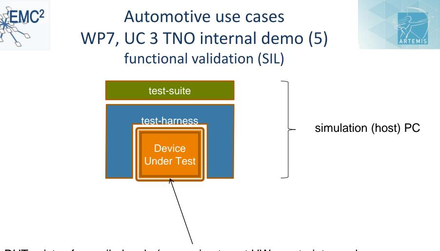
DUT exists of compiled code (presuming target HW constraints, such as fixed point parameters, target platform process scheduling, etc.)
