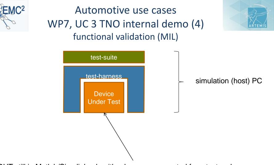
DUT still in Matlab/Simulink; algorithm however separated from test code
