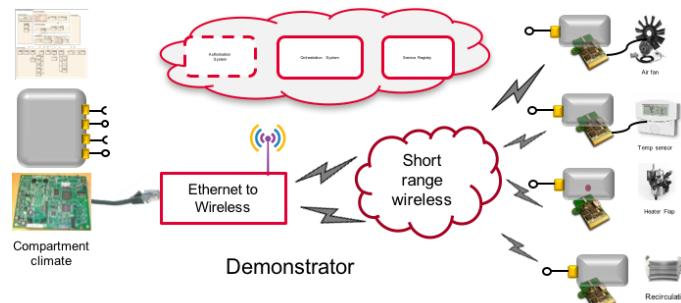
Figure 11: Multi-core ECU for climate control with SOA and wireless sensors and actuators
