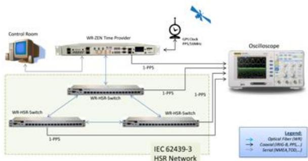
Figure 24: Time transfer fault tolerant system in HSR network
