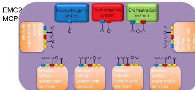
Figure 10: Diagram of an Arrowhead Framework local cloud with its three core services and other application services
