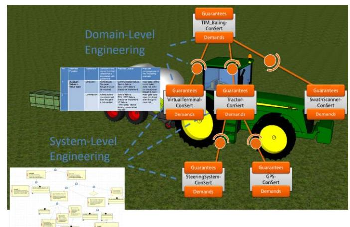
Figure 31: Example for run-time qualification/certification (FhG IESE ©); A tractor with various implements from different providers – do safety requirements hold?
