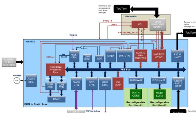
Figure 20: Reliable and Self-Healing DRM architecture diagram
