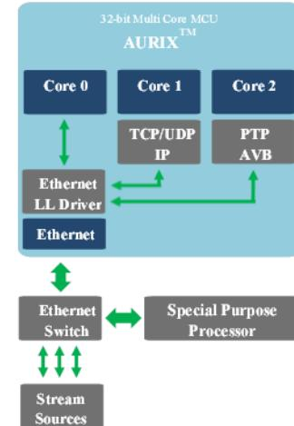
Figure 7: Infineon setup for the safe handling of mixed-critical communication
