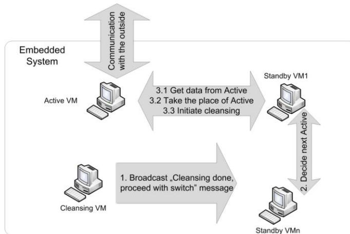
Figure 29: Multiple Virtual Machines to maintain secure system status
