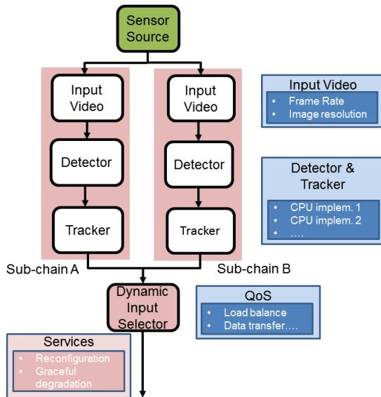
**Figure 26: Technical implementation of a passenger tracking application based on the proposed computer vision architecture. The Dynamic Input Selector (DIS) activates either sub-chain A or B depending on the current QoS**
