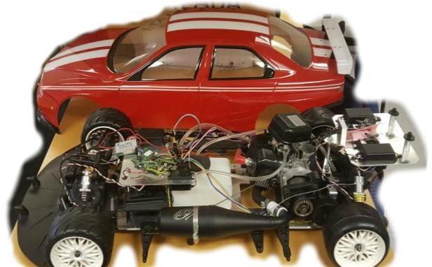
Figure 13: 1/5 scale model car with independent brakes
