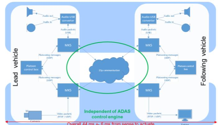
Figure 8: Presented by NXPNL setup with WiFi-p subsystem with mixed criticality data-streams (4 antennas/channels offer redundant messaging, bi-directional audio and video, ETSI standards compliance, diagnostics and security)
