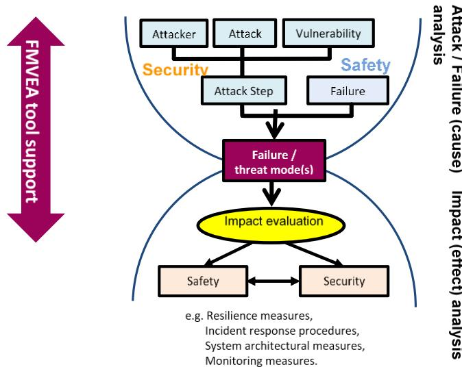
*Figure 27: Tool concept for partially automated model-based EMVEA*
