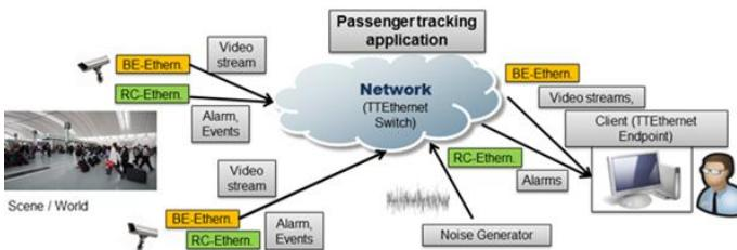
Figure 22: Measuring waiting time by utilising a deterministic network of cameras, server and client
