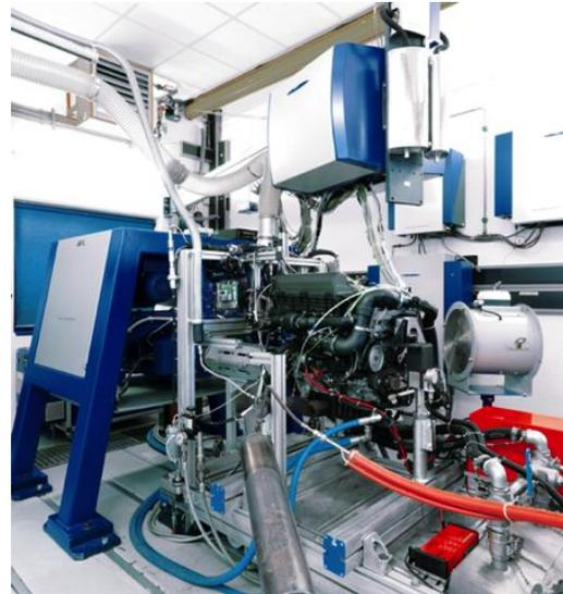
Figure 19: Engine Test Bed
