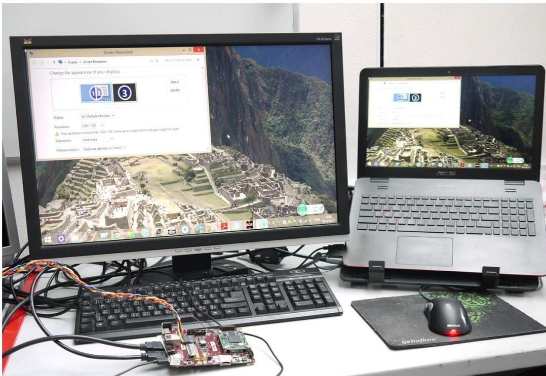
Figure 28: Sundance EMC<sup>2</sup>-DP board with the HDM-IN HDMI-OUT application demo
