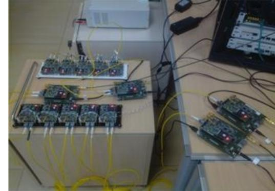
Fig A: Timing scalability jitter and QoS test using a daisy-chain setup with White Rabbit
