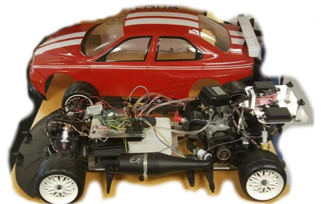
Figure 13: 1/5 scale model car with independent brakes
