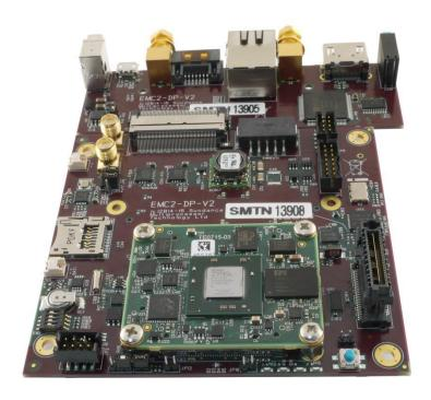
$\label{eq:Figure 1: The EMC} \textbf{EMC}^2 \ showing \ the \ Stackable \ PCIe/104 \ OneBank \ Connector \ and \ the \ Cable-less \ I/O \ board \ High-Resolution \ \underline{\textbf{download here}}$
