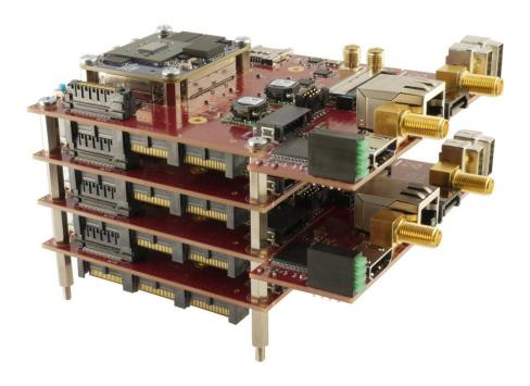
$\begin{tabular}{ll} Figure 2: EMC^2 stacked, using the PCI Express Lanes, to provide 8x ARM9 CPU Cores \\ High-Resolution \underline{download\ here} \end{tabular}$
