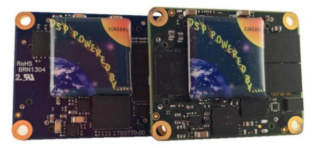
Figure 5: The 40mm x 50mm SoM Module for EMC<sup>2</sup> with Xilinx Zynq SoC, Artix-7 or Kintex-7 High-Resolution <u>download here</u>
