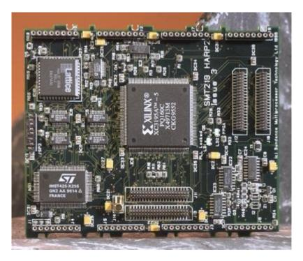
Figure 3: HARP-2 fitted onto a TRAM Module w. a 32-bit Inmos T425 CPU and a Xilinx XC3195 FPGA
