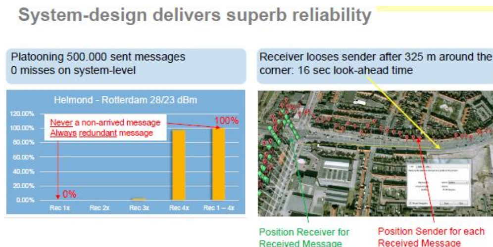
Figure 5: Reliability of wireless communication subsystem in first on the road tests
