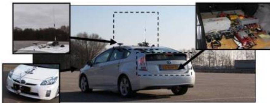
Figure 9: Instrumentation of TNO carlabs vehicle
