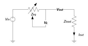
Fig. 1.2 Block Diagram of Linear Voltage Regulator
