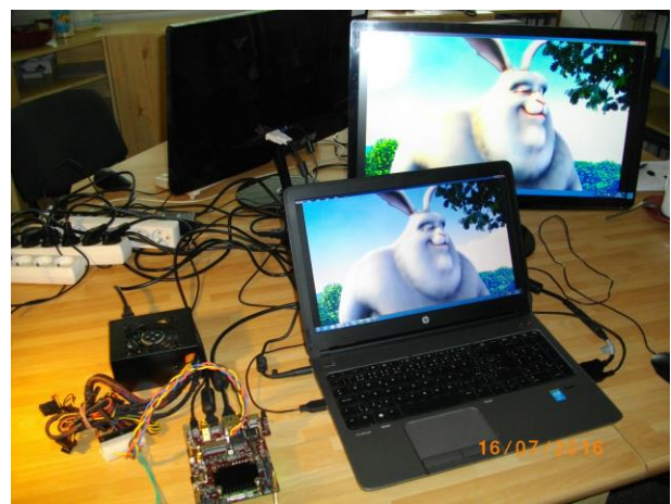
Figure 28 Standalone EMC2-DP-V2 platform with 3x (8xSIMD) EdkDSP (detailed view in left) and Full HD motion detection algorithm accelerated in HW (right).
