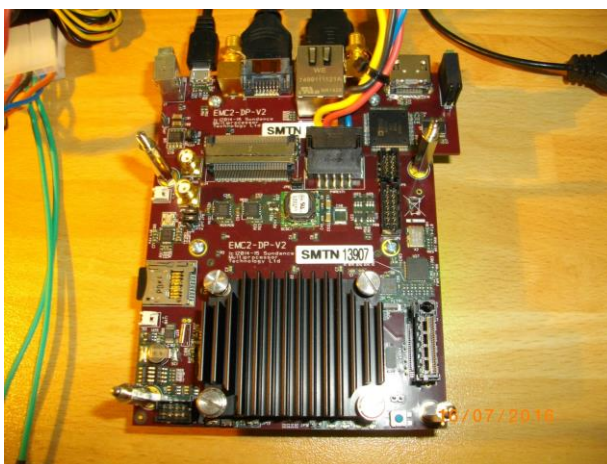
Figure 28 Standalone EMC2-DP-V2 platform with 3x (8xSIMD) EdkDSP (detailed view in left) and Full HD motion detection algorithm accelerated in HW (right).
