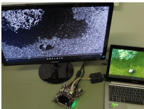
Figure 29: Edge-detection running on Sundance EMC2-DP with ZYNQ 7Z015-1I System on Module
