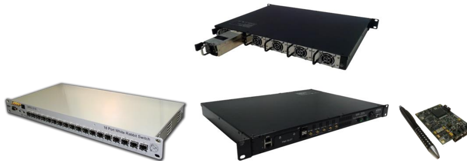
Figure 7: WR-Switch, WR-ZEN (Zynq architecture) and WR-LEN (node based on Artix FPGA).
