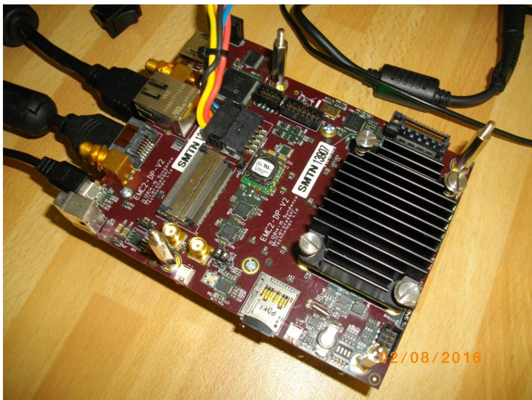
Figure 5: EMC2-DP-V2 platform with Zynq xc7z030-1I device and 3xEdkDSP accelerator
