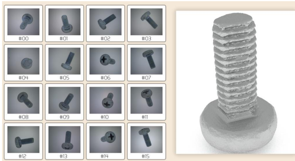
Figure 38: Quality control by 3D inspection
