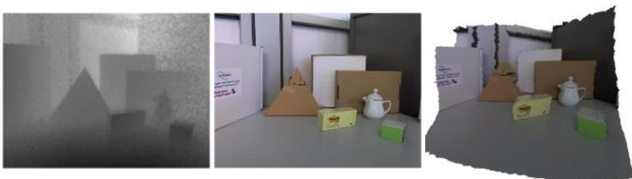
Figure 14: Time-of-Flight 3D imaging (left: low resolution ToF image; center: high resolution RGB image; right: fusion result of low resolution ToF and high resolution RGB image)
