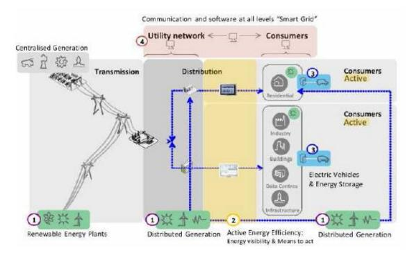
Figure 7: Smart Grid concept
