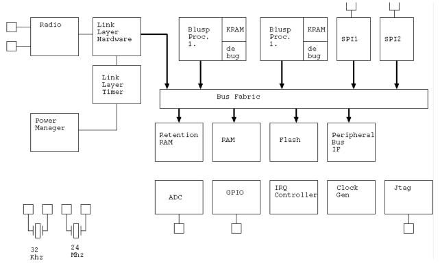
Figure 6: Demonstrator block diagram
