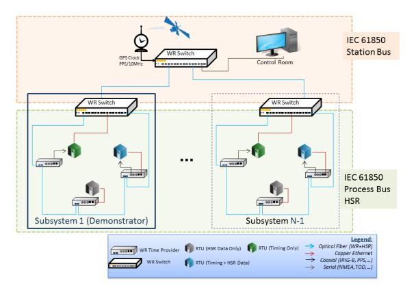
Figure 8: Demonstrator to be presented in the use case Synchronized low-latency deterministic networks
