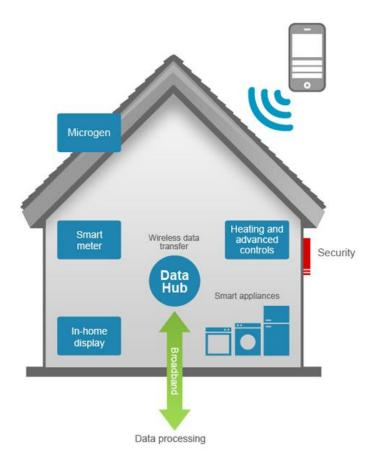
Figure 4: Autonomous smart home demonstrator
