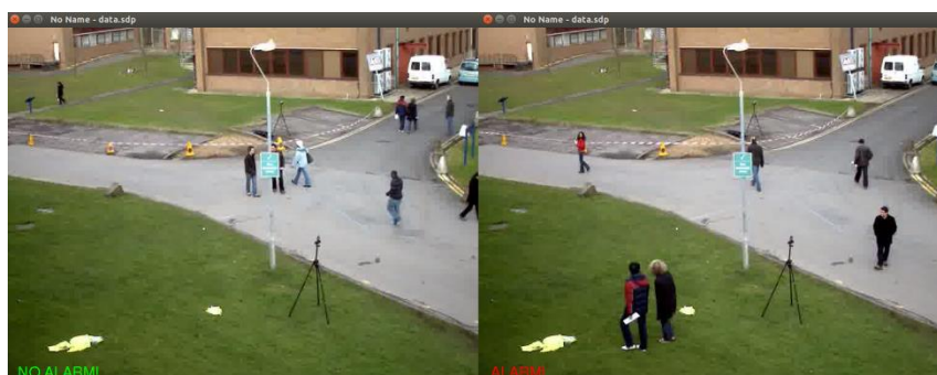
Figure 5: An alert is thrown if a person enters the lawn (right image).
