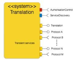
Figure 7: The Translator system and its produced and consumed services.
