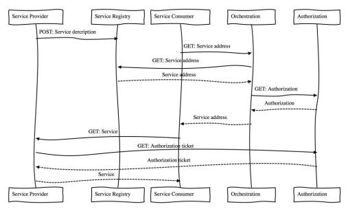
Figure 5: Simplified sequence diagram example of messages exchange in an Arrowhead Framework Local Cloud.
