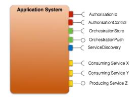
**Figure 6:** A System is capable of consuming the Framework mandatory core Services and will produce and/or consume one or more services.
