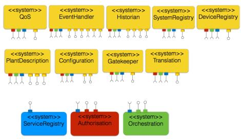
Figure 2: Mandatory core and Support Systems of the Framework.
