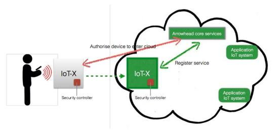
Figure 9: A two-way hardware authentication in conjunction with the core Authorization service.
