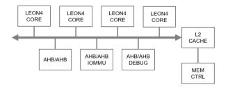
Figure 1 - Schematization of the NGMP architecture
