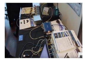
Fig B: Heterogeneous Time distribution with White-Rabbit and IRIG-B in a daisy-chain setup and a redundant HSR ring
