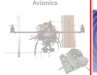
Flight Control Computer for a Remotely Piloted Aircraft **Goal**: *Executes safety-, mission- and non-critical applications on the same multi-core execution platform.* **Criticalities**: *safety- and mission-critical* **Extra-functional properties**: *hard real-time, power, temperature, reliability*
