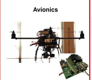
Flight Control Computer for a Remotely Piloted Aircraft **Goal**: *Executes safety-, mission- and non-critical applications on the same multi-core execution platform.* **Criticalities**: *safety- and mission-critical* **Extra-functional properties**: *hard real-time, power, temperature, reliability*
