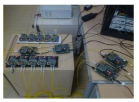
Fig A: Timing scalability jitter and QoS test using a daisy-chain setup with White Rabbit
