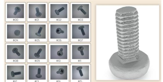
Increased overall inspection performance by 300%: With OpenMP parallelization and an execution platform composed of 2 processors, 16 cores and multithreading capabilities a reduction of computation time from 24.563 milliseconds to 7.996 milliseconds is achieved by exploiting coarse parallelism and thus decreasing latency.
