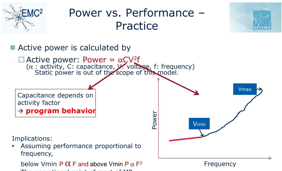
The operational point of most of MP systems is around Vmin
