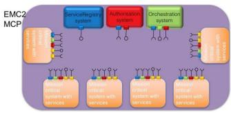
Figure 10: Diagram of an Arrowhead Framework local cloud with its three core services and other application services
