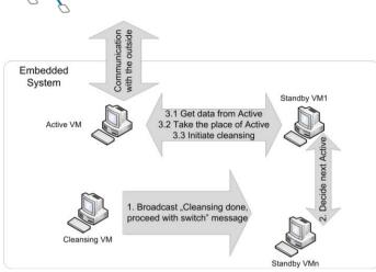
Figure 29: Multiple Virtual Machines to maintain secure system status
