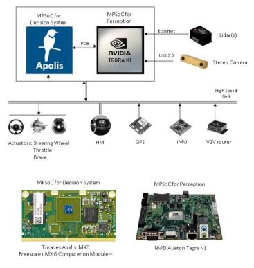
Figure 15: HW architecture of the MPSoC for UC T7.2
