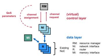
*Figure 6: Structure of the SoC system with the global and dynamic arbitration introduced by TUBS*
