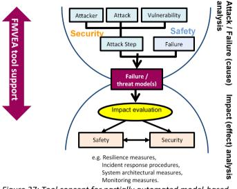
Figure 27: Tool concept for partially automated model-based FMVEA
