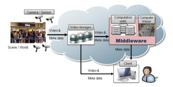
Figure 25: Airport surveillance system with computing units extended by the proposed middleware. IP camera videos are streamed and centrally recorded as well as processed. Videos and Meta data are monitored by the operator on demand.
