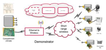
Figure 11: Multi-core ECU for climate control with SOA and wireless sensors and actuators
