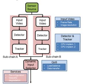
Figure 26: Technical implementation of a passenger tracking application based on the proposed computer vision architecture. The Dynamic Input Selector (DIS) activates either subchain A or B depending on the current QoS
