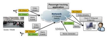
*Figure 22: Measuring waiting time by utilising a deterministic network of cameras, server and client*
