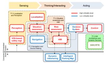
Figure 14: Functional architecture of the highly automated driving urban commuting use case
