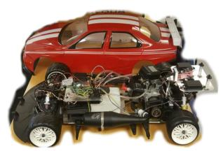
Figure 13: 1/5 scale model car with independent brakes
