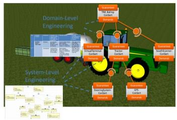
*Figure 31: Example for run-time qualification/certification (FhG IESE ©); A tractor with various implements from different providers – do safety requirements hold?*
